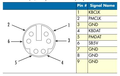
Table 13. J7: Mouse(PS/2 Mouse) - 6-pin Mini-Din Connector
